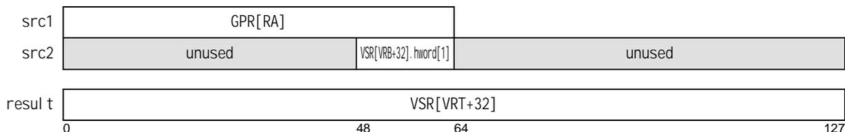
**Vector Insert Word from VSR using GPR-specified Left-Index VX-form**
