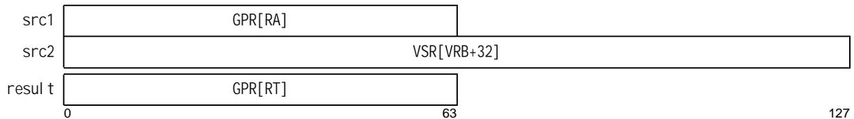
**Vector Extract Unsigned Halfword to GPR using GPR-specified Left-Index VX-form**
