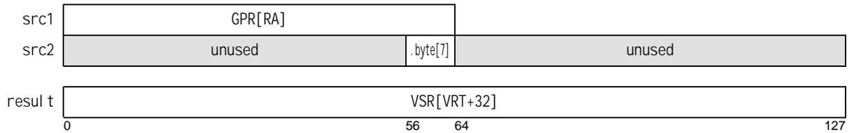
**Vector Insert Halfword from VSR using GPR-specified Left-Index VX-form**
