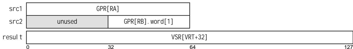
**Vector Insert Doubleword from GPR using GPR-specified Left-Index VX-form**
