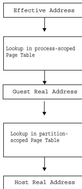
**Figure 26. Address translation overview, Radix on Radix**
