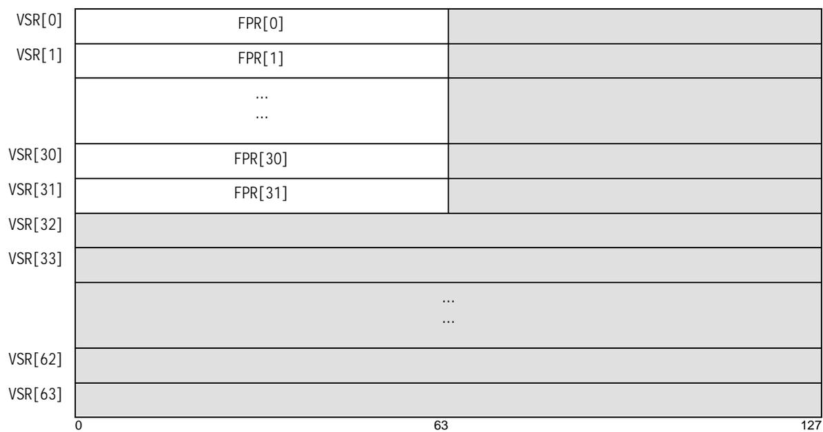
Figure 107. Floating-Point Registers as part of VSRs
