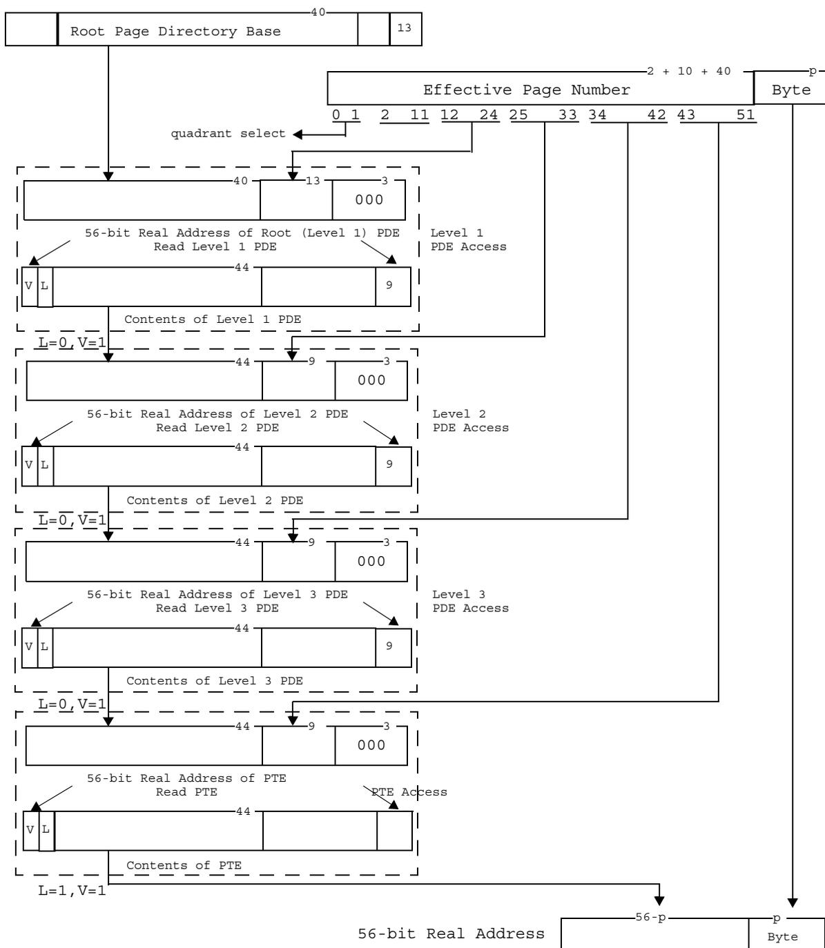
Figure 34. Four level Radix Tree walk translating a 52b EA with NLS=13 in the root PDE and NLS=9 in the other PDEs.
