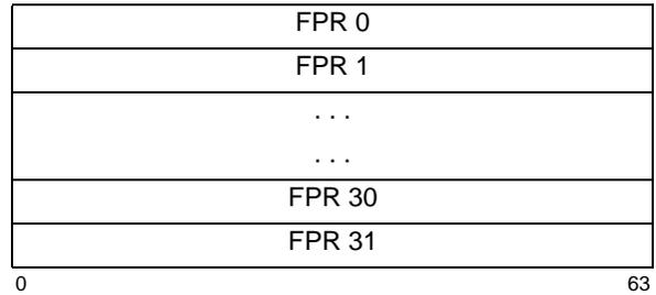
Figure 45. Floating-Point Registers
