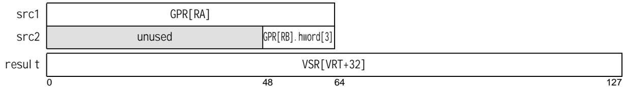
**Vector Insert Word from GPR using GPR-specified Left-Index VX-form**
