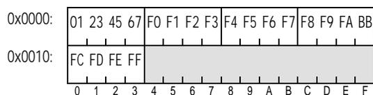
**Figure 127.** Process to store unaligned quadword to Big-Endian storage using Store VSX Vector Word\*4 Indexed
