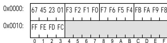
**Figure 128.** Process to store unaligned quadword to Little-Endian storage Store VSX Vector Word\*4 Indexed
