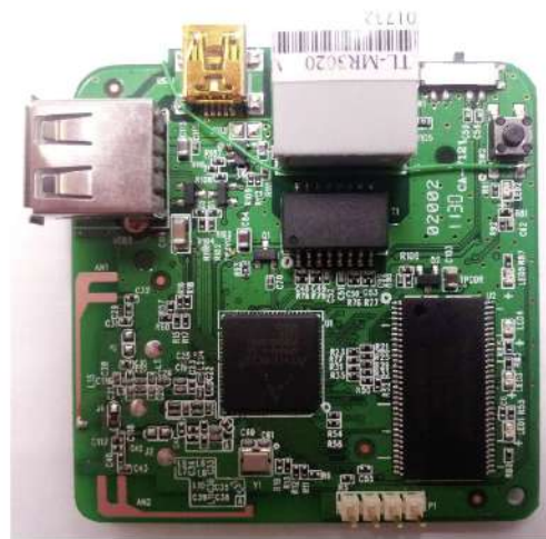
Figure 6: modified MR-3020 Top View
