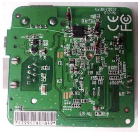
Figure 5: modified MR-3020 Bottom View
