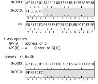
Figure 127.Process to store unaligned quadword to Little-Endian storage Store VSX Vector Word\*4 Indexed
