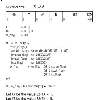
For each vector element i from 0 to 3, do the following. Let src be the single-precision floating-point operand in word element i of VSR[XB].
