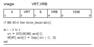
For each integer value i from 0 to 3, do the following. The sum of the one's-complement of the signed integer in word element i of VR[VRB] and 1 is placed into word element i of VR[VRT].
