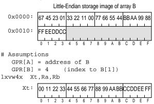
Figure 125.Process to load unaligned quadword from Little-Endian storage Load VSX Vector Word\*4 Indexed
