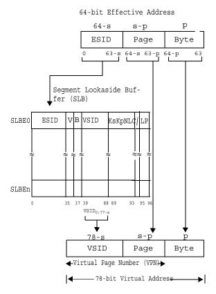
Figure 26. Translation of 64-bit effective address to 78 bit virtual address
