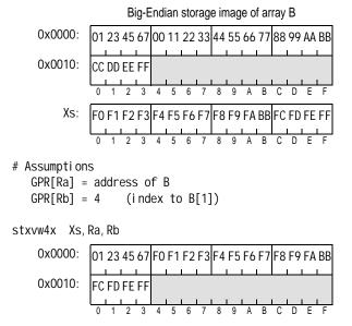
Figure 126.Process to store unaligned quadword to Big-Endian storage using Store VSX Vector Word\*4 Indexed
