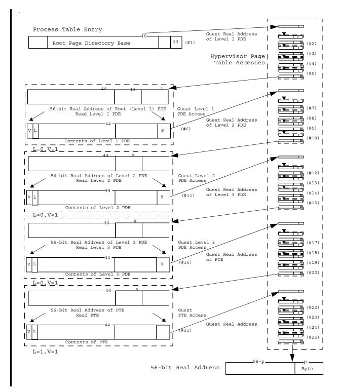
Figure 36. Radix on Radix Page Table search for a 52-bit EA depicting memory reads 1-24 numbered in sequence
