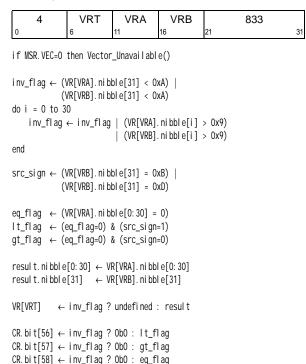
The decimal value in VR[VRA] is placed into VR[VRT] with the sign code of the decimal value in VR[VRB].
