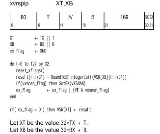
For each vector element i from 0 to 3, do the following. Let src be the single-precision floating-point operand in word element i of VSR[XB].
