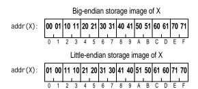
Loading a vector of 8 halfword elements from Big-Endian storage in VSR[XT] using *Ixvh8x*, retaining left-to-right element ordering.
