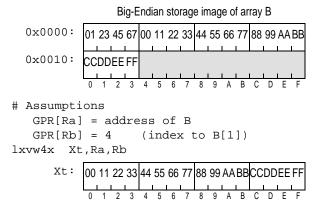
Figure 124.Process to load unaligned quadword from Big-Endian storage using Load VSX Vector Word\*4 Indexed
