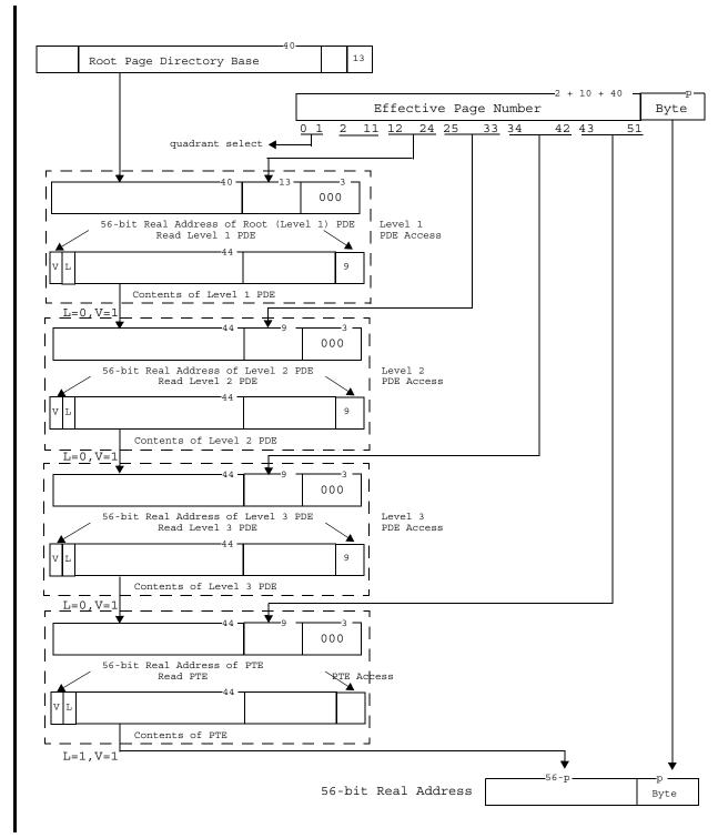
Figure 33. Four level Radix Tree walk translating a 52b EA with NLS=13 in the root PDE and NLS=9 in the other PDEs.
