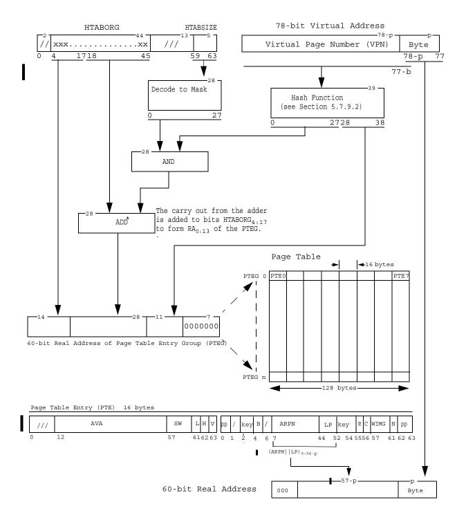
Figure 30. Translation of 78-bit virtual address to 60-bit real address
