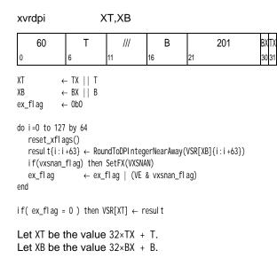
For each vector element i from 0 to 1, do the following. Let src be the double-precision floating-point operand in doubleword element i of VSR[XB].
