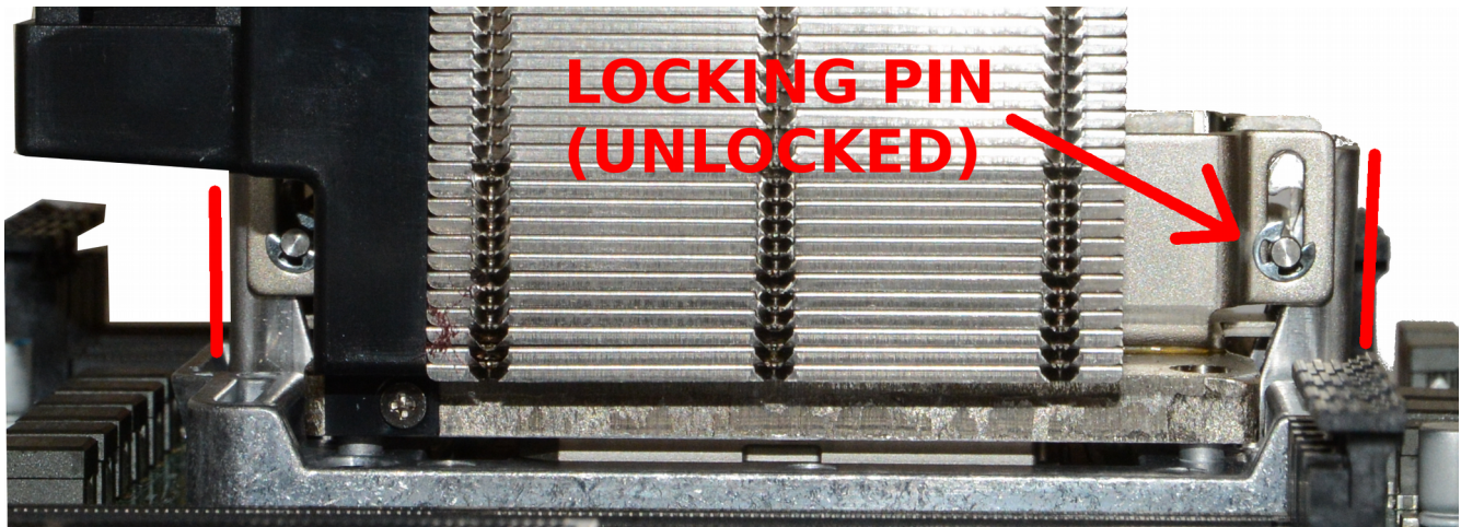
Illustration 2: Correct Retention Mechanism Prong Alignment (Unlocked)
