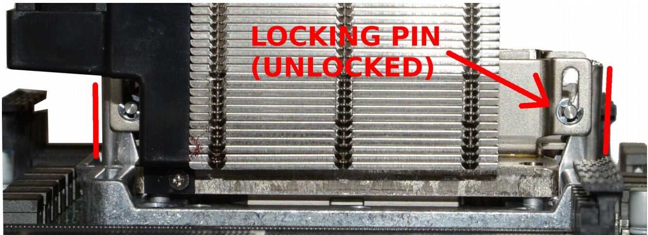
Illustration 2: Correct Retention Mechanism Prong Alignment (Unlocked)
