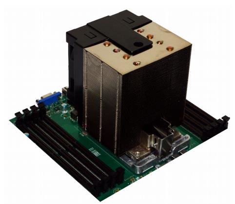
Illustration 6: Align Pins and Place Heatsink on CPU
