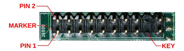
Illustration 8: Dual Row Header with Annotated Pins, Marker, and Key
