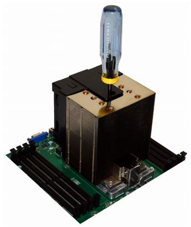
Illustration 7: Tighten Retention Scew until Hard Stop
