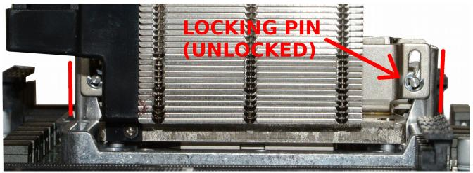
Illustration 2: Correct Retention Mechanism Prong Alignment (Unlocked)
