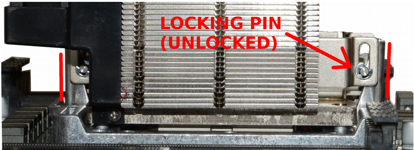
Illustration 2: Correct Retention Mechanism Prong Alignment (Unlocked)
