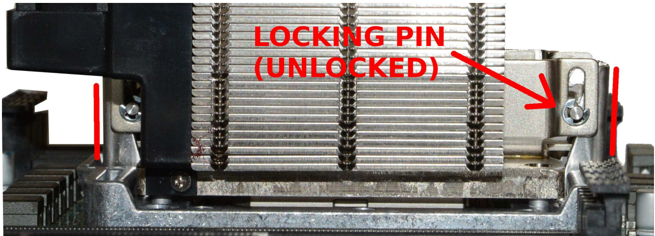
Illustration 2: Correct Retention Mechanism Prong Alignment (Unlocked)
