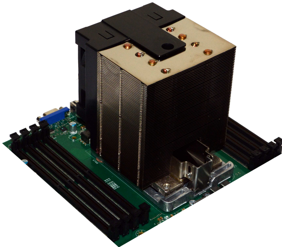
Illustration 6: Align Pins and Place Heatsink on CPU
