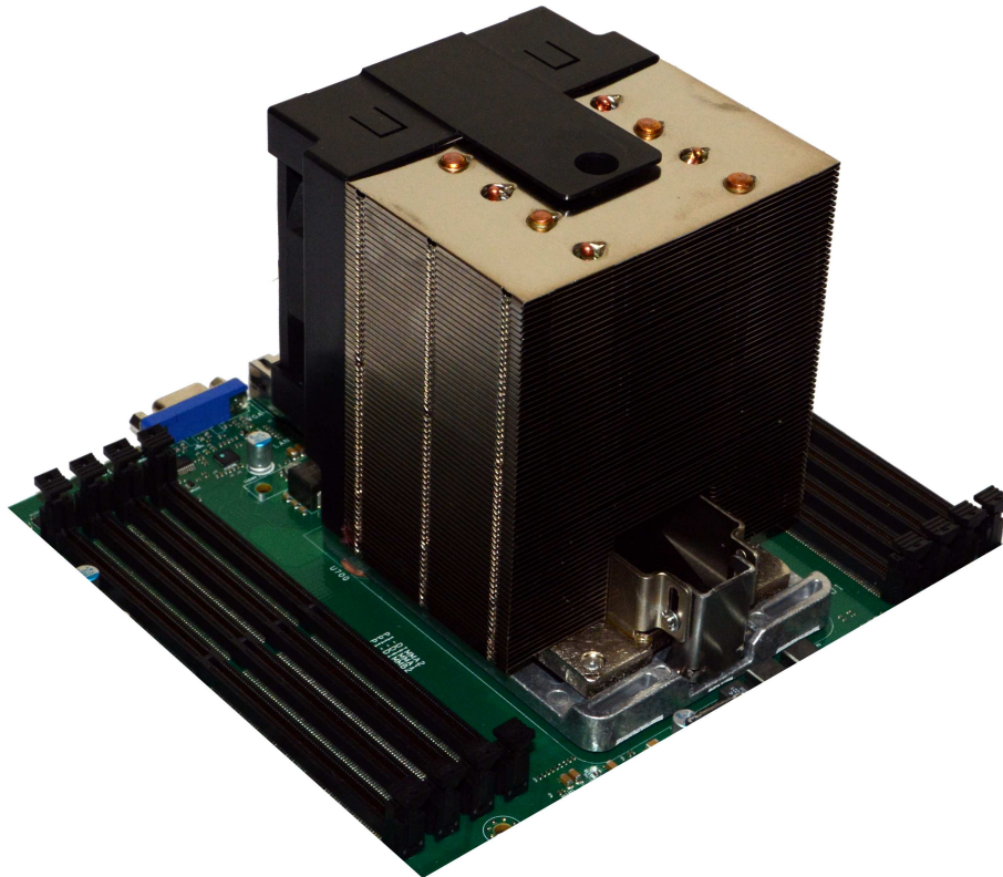
Illustration 6: Align Pins and Place Heatsink on CPU
