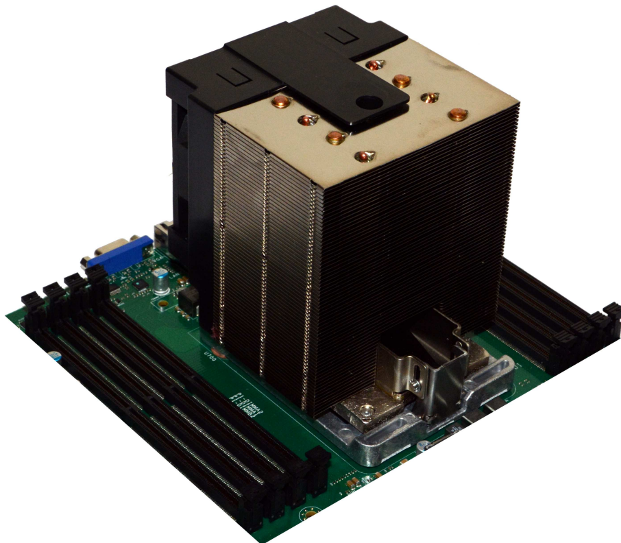
Illustration 6: Align Pins and Place Heatsink on CPU
