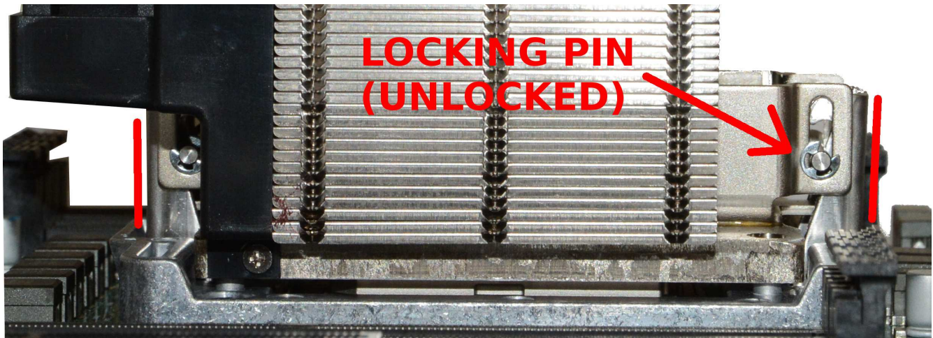
Illustration 2: Correct Retention Mechanism Prong Alignment (Unlocked)
